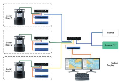
A typical multi-head network - Up to 10 sonar heads can be integrated into a single command workstation, with each head requiring its own sonar processor
