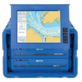
Processor and Software Pulse compression, beam forming and automatic detection and tracking (ADT) are carried out in two high performance PCs installed in a rugged case.
